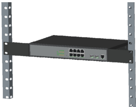
Figure 2-2 Install switch to the rack
