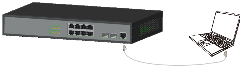
Figure 2-5 Connect configuration cable
