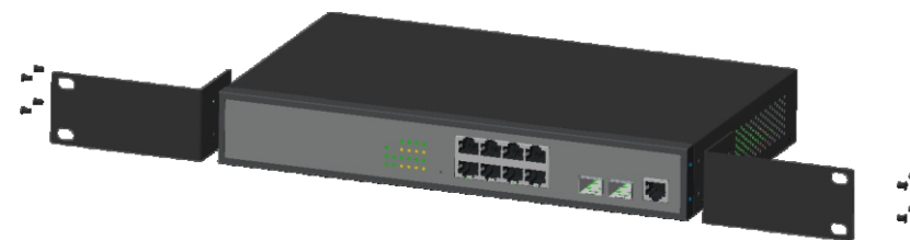
Figure 2-1 Install hangers diagram
