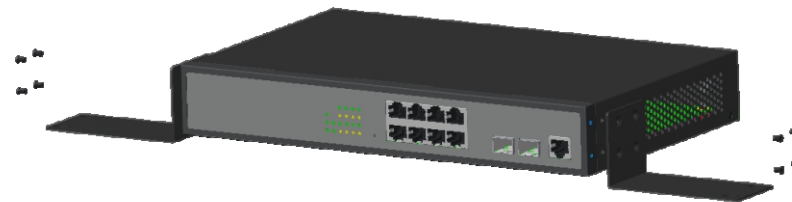
Figure 2-3 Hangers installation diagram
