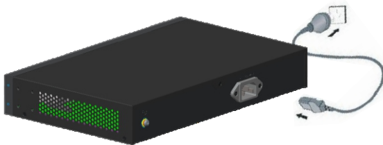
Figure 2-6 Connect power cable
