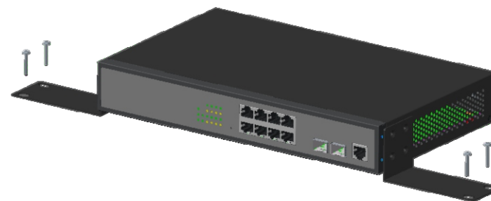
Figure 2-4 Fix the switch on wall
